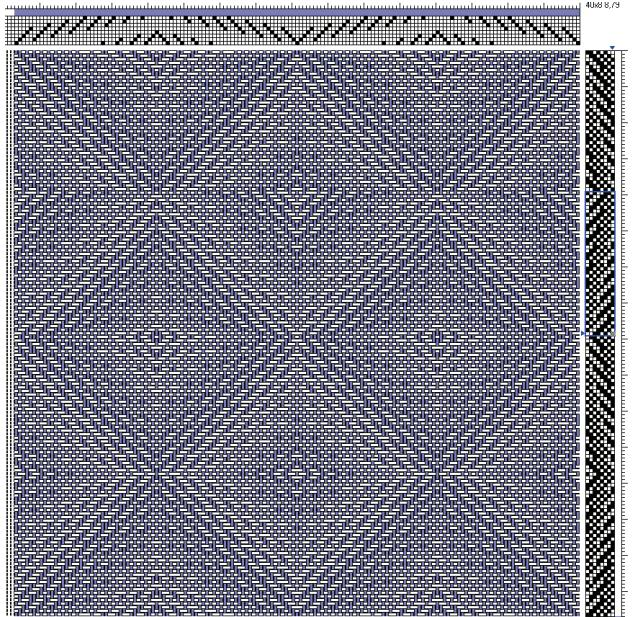
Change the liftplan as desired. Just part of the liftplan was ‘wrapped’ to produce a new design.
